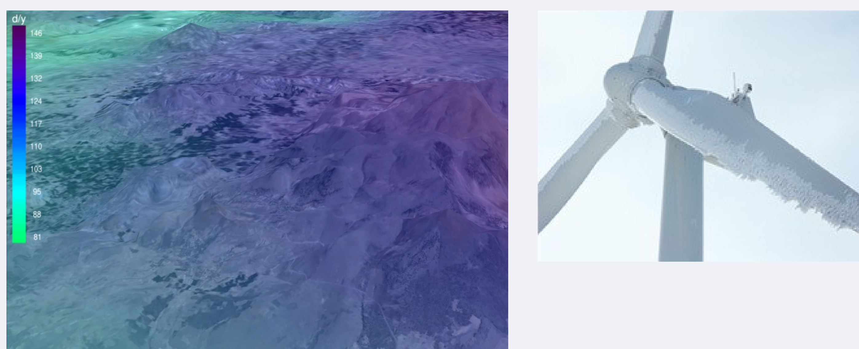
(1) This figure shows the number of days per year below a temperature threshold based on Vortex WRF 3km temperature output driven by NCEP/CFS Reanalysis 0.5 degrees data.
